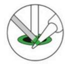
With the iron touching feed solder to the joint
