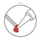
Don't glob solder onto the iron and then try to apply
